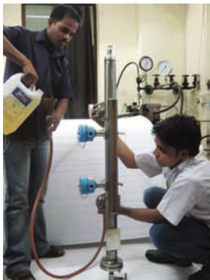
Low CCD of 350 mm with special specific gravity float of 0.4 being tested with kerosene for refinery application.
