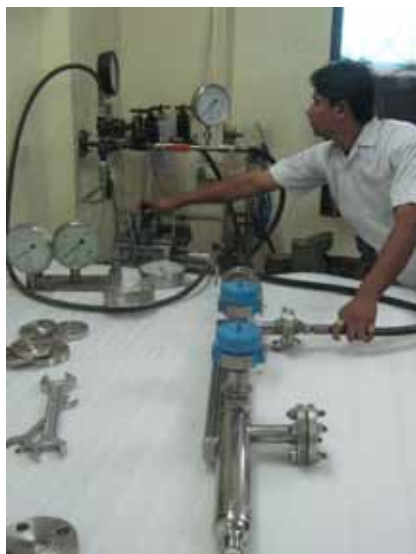
Hydrotest and helium leak test for magnetic level gauge
