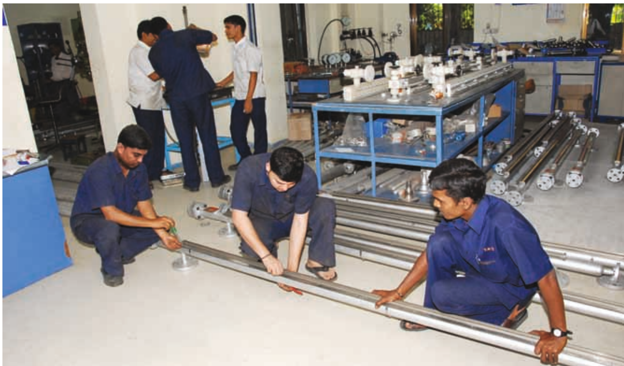
Assembly of magnetic flappers on magnetic level gauge. Flappers are with 3.5mm thickness rolling at 180 deg change on the float sensing the level
