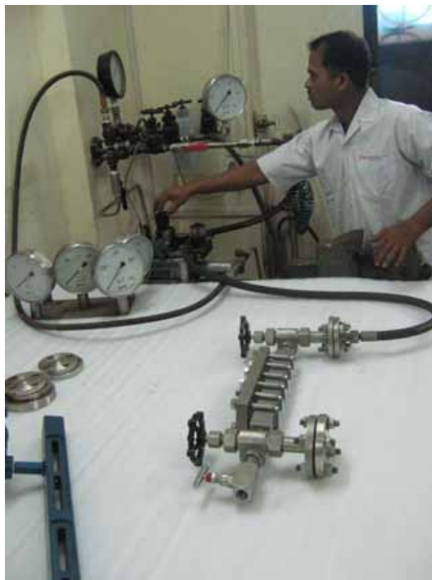
Hydro test bench and calibration test bench applicable with helium leak test for gauges for perfect tight sealing feature
